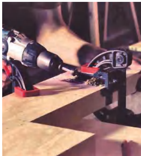
▲ Pic.9 Screwing the boards together, to provide added strength
